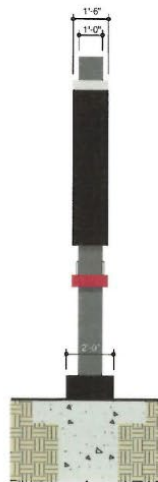
2 Sign Type M2 - West Elevation Scale: 1/4" = 1'-0"
